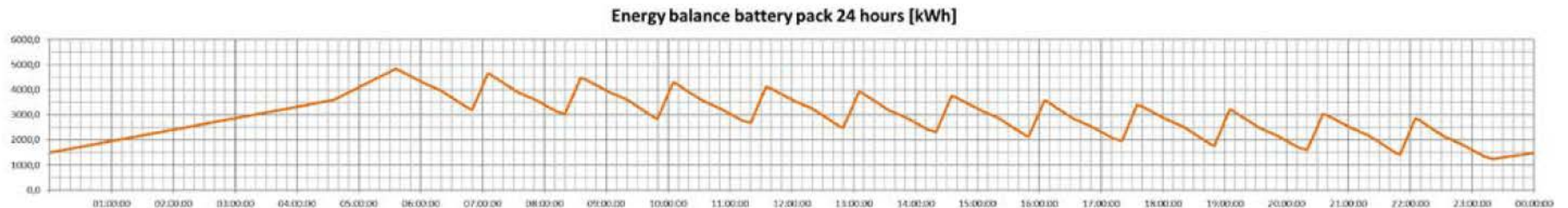
Figure 4.1.1 Energy balance or battery capacity used during a full day and night of operation with 12 single trips or 6 roundtrips for one E-Ferry Twin. Compiled by EMK.
